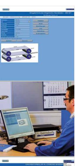
We developed our Belt Manager Software specially for the application of steel belts in the wood processing industry. This makes it possible for belt users to store and evaluate all inspection data of their steel belts.
